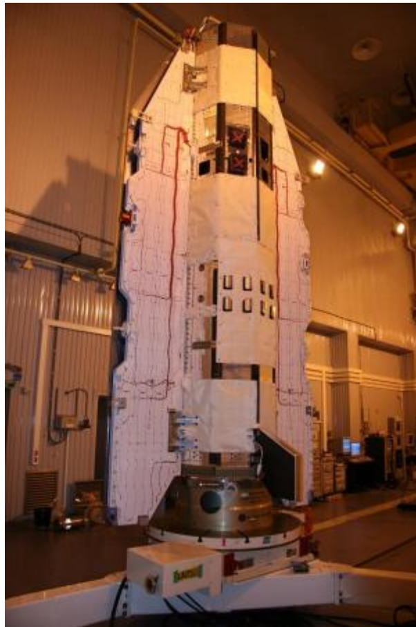
GOCE positioned on the rotary table for alignment check, during launch campaign at the Plesetsk Cosmodrome. (Credit: ESA)
